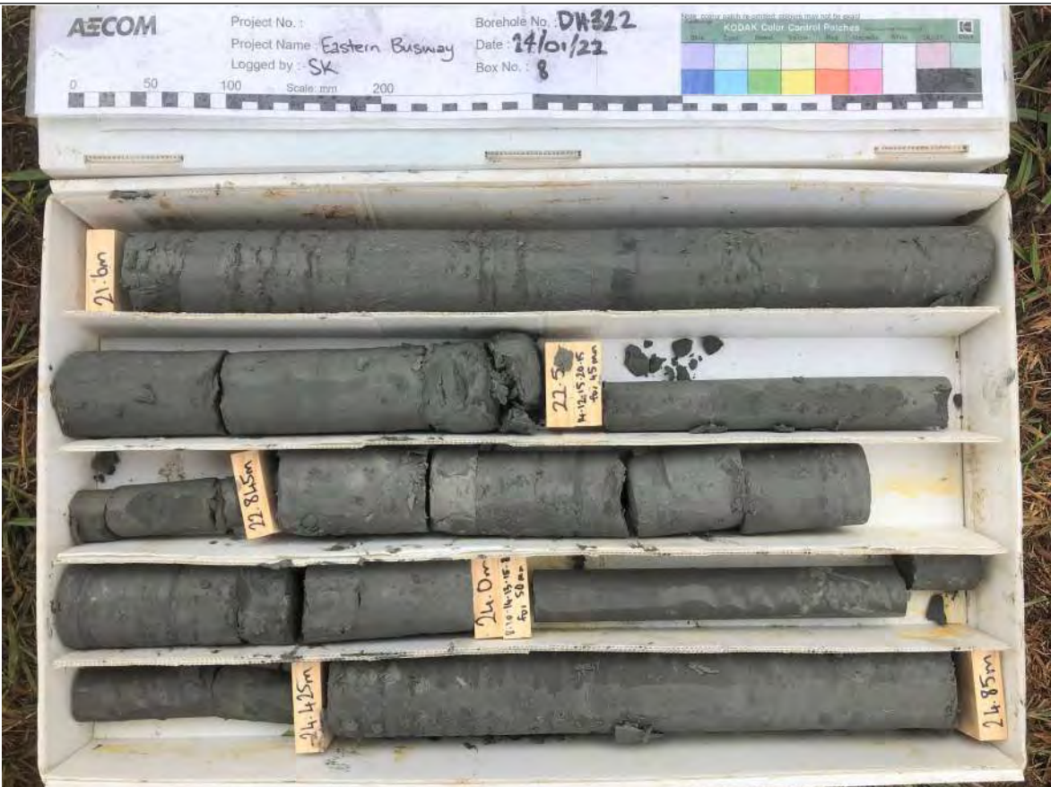
Box: 8 of 9 - Depth: 21.60m to 24.85m of 27.00m
