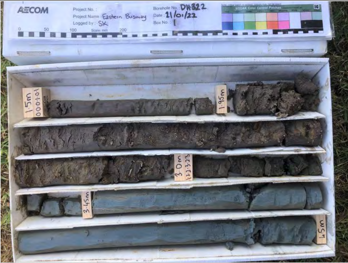
Box: 1 of 9 - Depth: 01.50m to 04.50m of 27.00m
